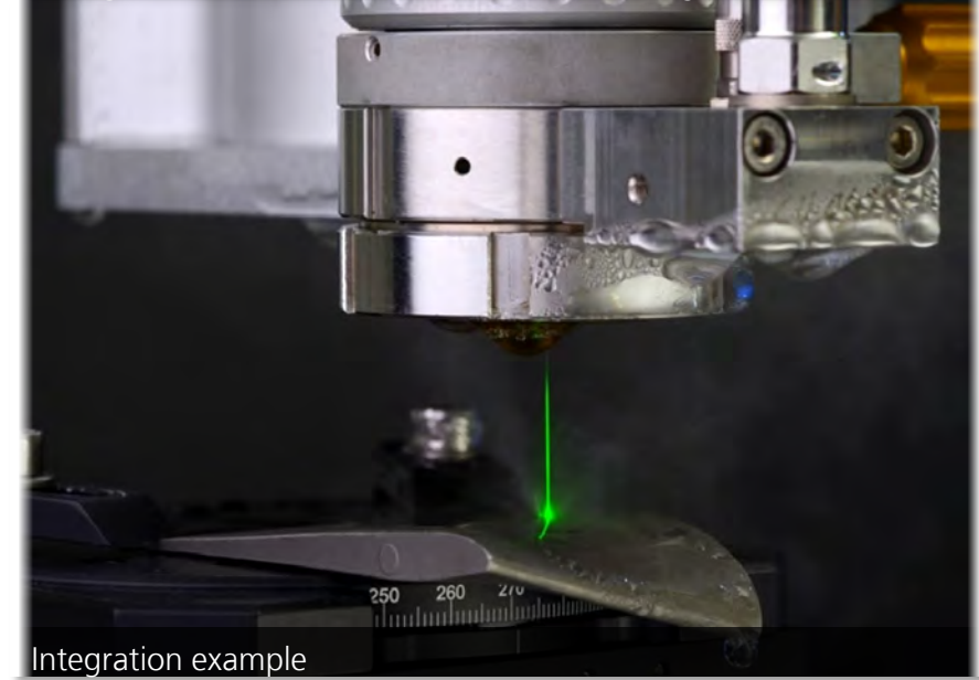
Topographic measurement of a workpiece using OCT
