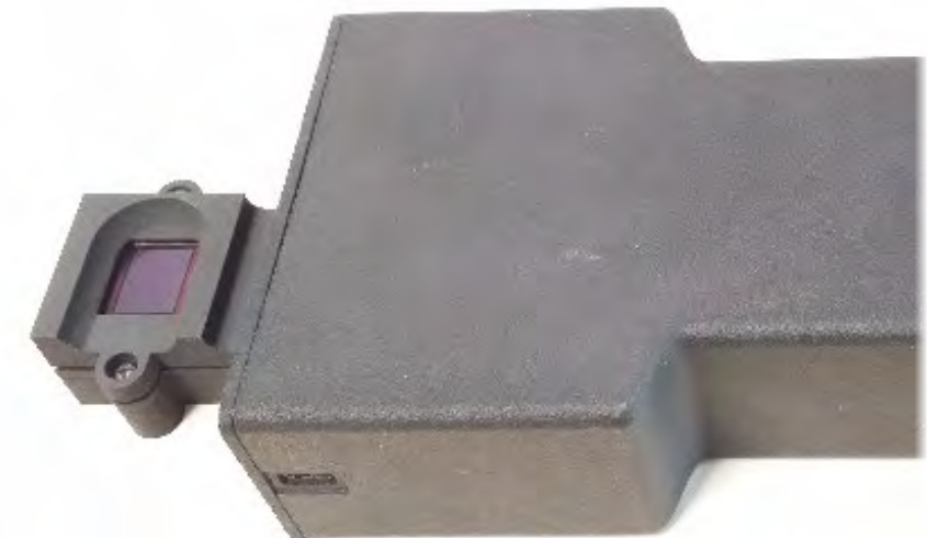
Display with finger rest and control electronics
